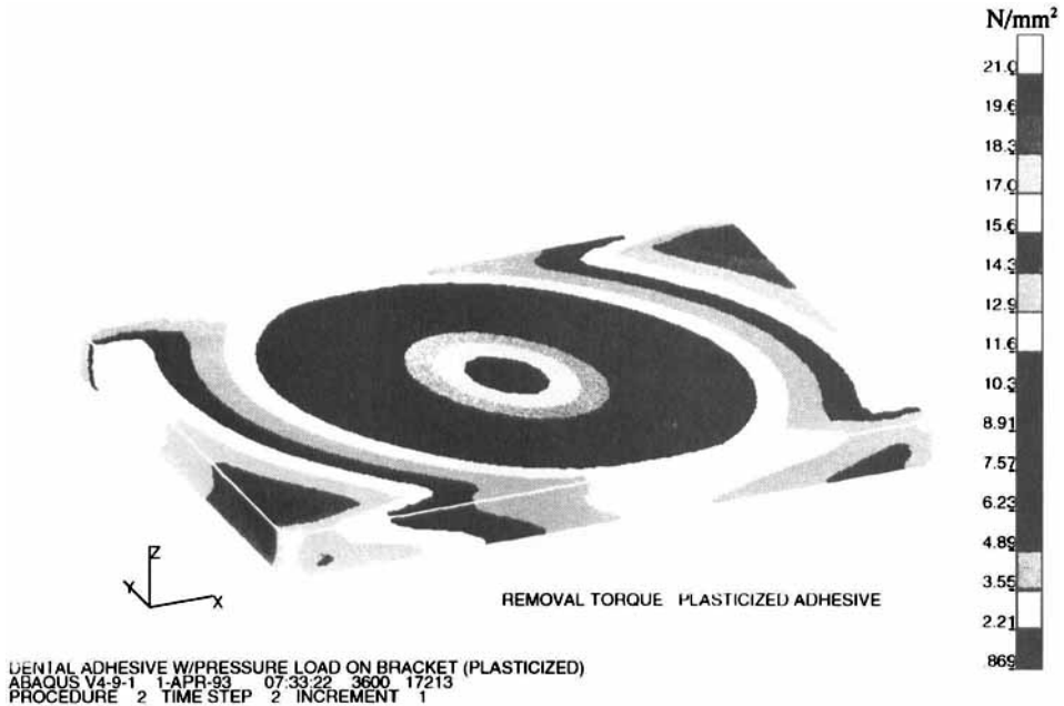
FIGURE 3 FEM von Mises stress distribution for the plasticized region applying typical torque removal force conditions (simulating "removal"). See Color Plate II.
